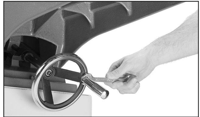
Figure 12. Securing the handwheel handle.
